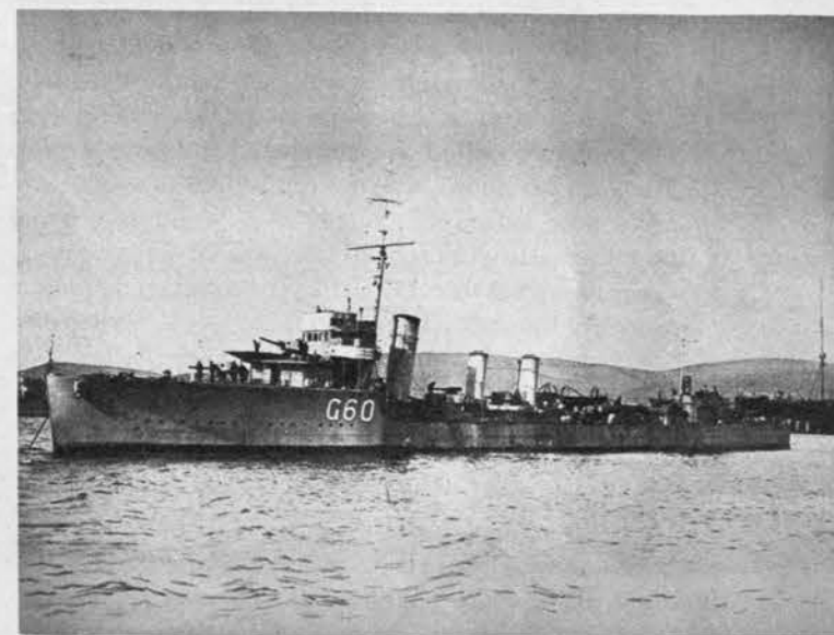
SUPERFIRING GUNS , greatest single step in destroyer evolution, were introduced in 1916 by Seymoure Class flotilla leaders, named for famous British naval officers. This is the Anzac, first Australian leader.
